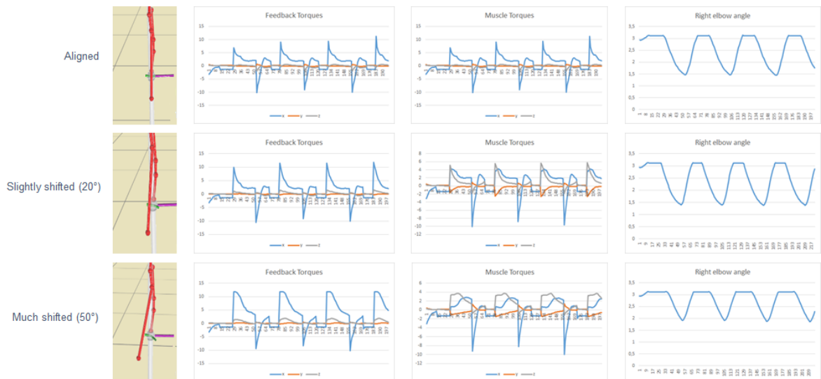
Figure 10: Comparison of three different configurations of the biceps moment arm and the elbow's x -axis DOF. From left to right: the placement of the muscle (in red) with the DOF in purple and the moment arm in green, the Feedback Torques computed by the controller, the torques generated by the muscles and the angles in radians reached by the elbow. The recording frequency is 50 Hz.
